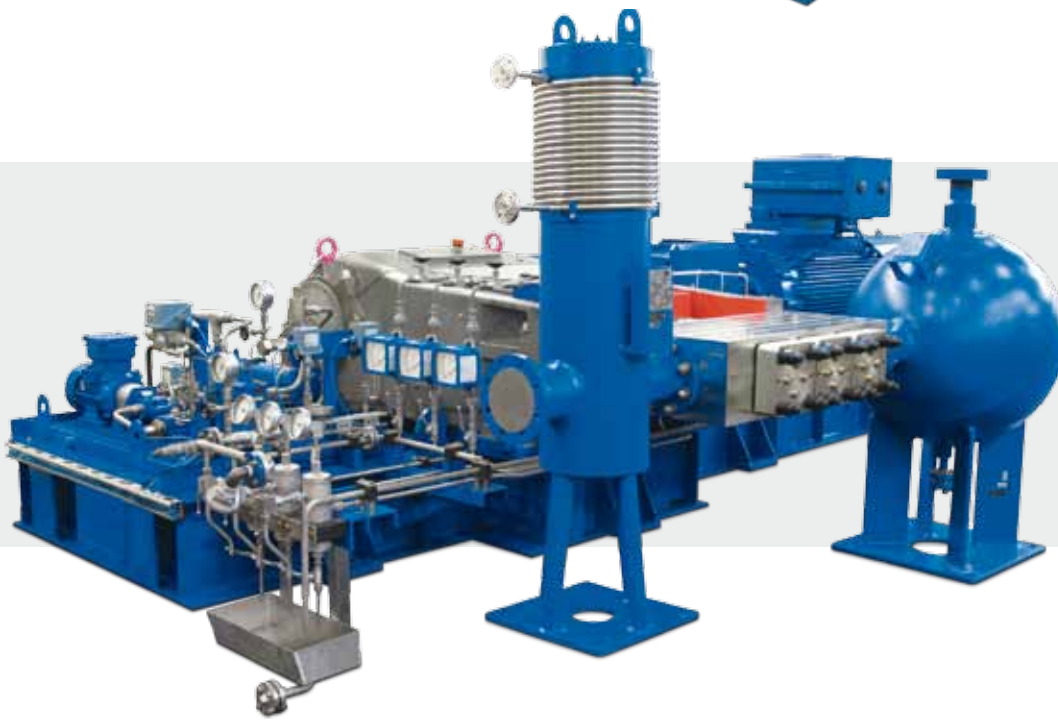
High-pressure pump unit KD823 for liquid NH 3 with partly heated pulsation damper, discharge ball resonator and lube oil system
