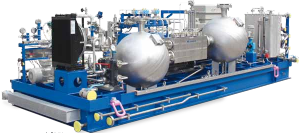
High-pressure pump unit P5-70 with suction and discharge sided resonators and lube oil system
